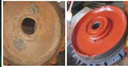
Rebuilding and ceramic coating against abrasion
