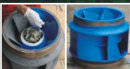
Ceramic coating with resistance to 240°C
