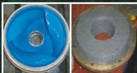
Rebuilding and ceramic coating against abrasion
